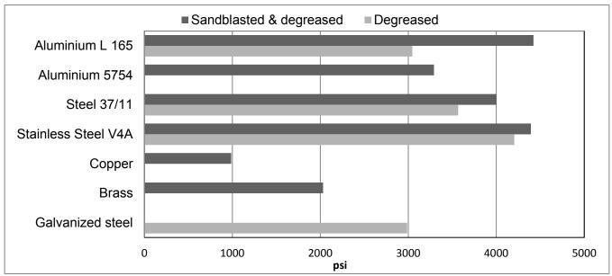
Notes: ARALDITE® 2050 is not suitable to bond copper or brass without surface preparation. Steels should not be abraded or sandblasted, better results are obtained with only degreasing.
