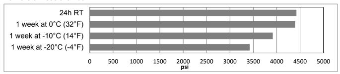
Average lap shear strengths (ASTM D1002) after application, bonding and curing under water (typical average values). Cured 24 hours under water at 23°C (73°F)
