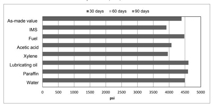
Lap shear strength (ASTM D1002) versus Cataplasma ageing (typical average values). Cure 24 hours at 23°C (73°F) – Cataplasma according to ISO 9142/E2. Tested at 23°C (73°F). Metals sandblasted and degreased / plastics abraded and degreased.
