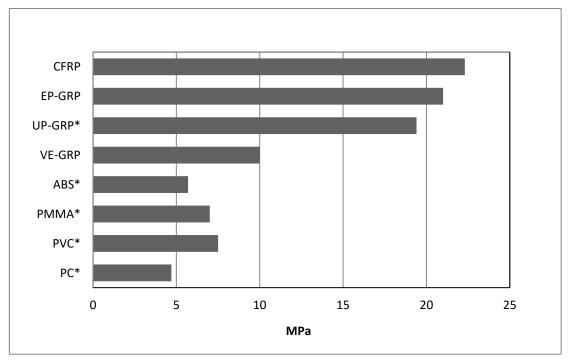
(\*): UP-GRP, ABS, PMMA, PVC, PC, substrate's failure or substrate's delamination failure observed.
