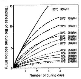
Relationship between curing speed and temperature/humidity
