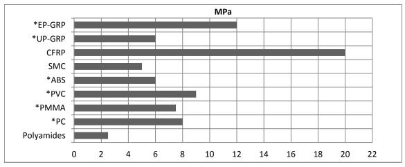
Average lap shear strengths of typical plastic-to-plastic joints (ISO 4587) (typical average values)
