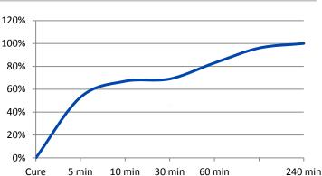
Heat Aging (aged at temp indicated and tested @ 22°C)
