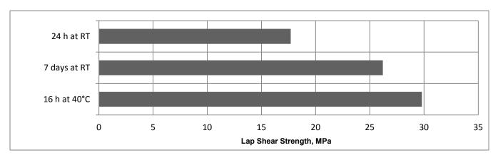
Average lap shear strengths of typical plastic-to-plastic joints (ISO 4587) (typical average values) Cured for 16 hours at 104°F (40°C) + 1 hour at 176°F (80°C) and tested at 73°F (23°C). Pretreatment -Lightly abraded and alcohol degreased.
